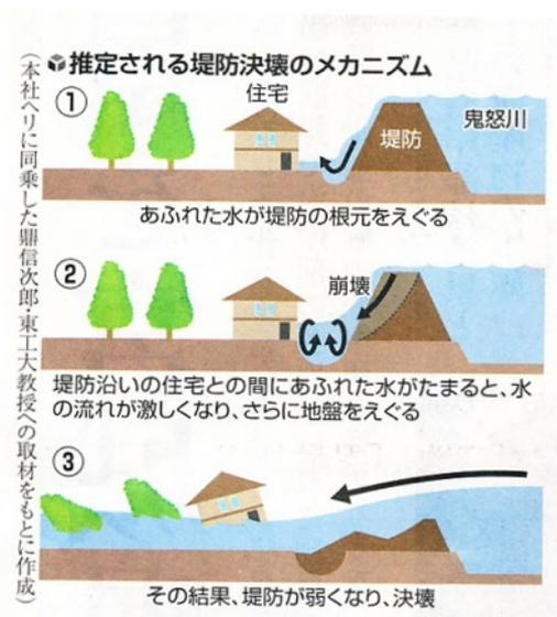
Figure 2: Mechanism of bank collapse due to water pressure effect demonstrated in a newspaper for the Kinu River flood, Sept. 2015 (by Prof. S. Kanae). Photo from Yomiuri Shinbun. Note that the style of erosion and rapid flow-in is very similar to that of the Tohoku tsunami, 2011.
